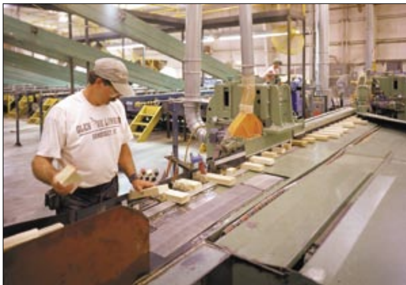
Defect-free blocks are positioned for finger-jointing into long, straight lengths for top-quality components.
